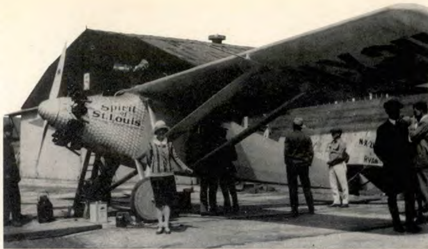
The aircraft, whose official designation was the Ryan M-2, was about the size of a single-engine Cessna or Piper and was literally nothing but a flying gas tank with wings.
